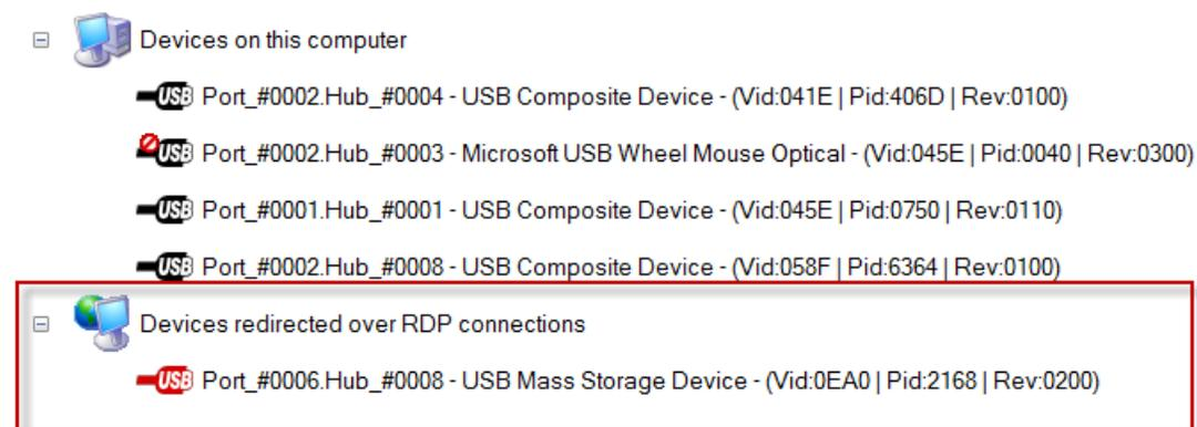
As shown in figure above those devices are listed which are connected locally and labelled separately which are redirected over RDP to the server.
